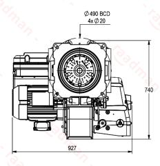
Suggested boiler flange diameter = 336 mm
