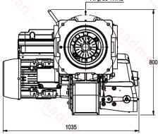
Suggested boiler flange diameter = 337 mm
