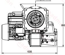
Suggested boiler flange diameter: ~337 mm
