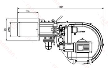
Suggested boiler flange diameter = 192 mm
