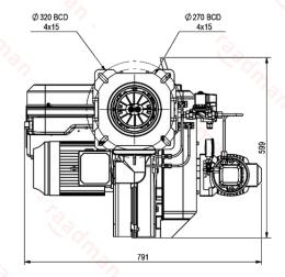
Suggested boiler flange diameter = 206 mm
