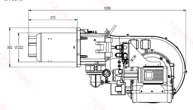
Suggested boiler flange diameter = 235 mm
