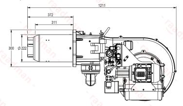
Suggested boiler flange diameter = 235 mm
