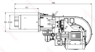
Suggested boiler flange diameter = 235 mm
