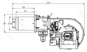
Suggested boiler flange diameter = 235 mm
