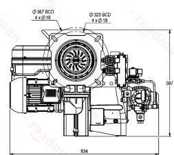
Suggested boiler flange diameter = 235 mm
