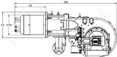
Suggested boiler flange diameter = 336 mm
