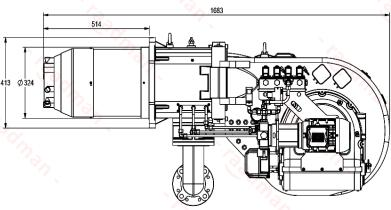
Suggested boiler flange diameter = 336 mm
