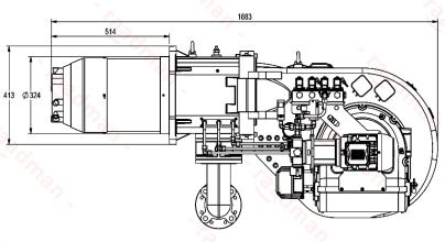
Suggested boiler flange diameter = 336 mm
