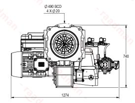
Suggested boiler flange diameter = 336 mm
