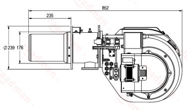
Suggested boiler flange diameter = 188 mm
