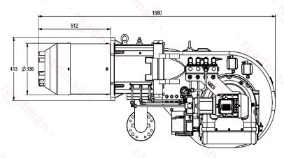
Suggested boiler flange diameter = 348 mm
