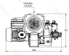
Suggested boiler flange diameter = 348 mm
