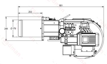
Suggested boiler flange diameter = 192 mm
