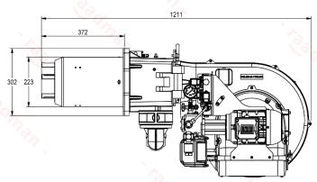
Suggested boiler flange diameter = 235 mm
