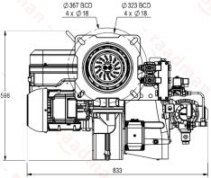
Suggested boiler flange diameter = 235 mm
