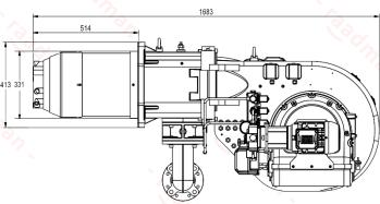
Suggested boiler flange diameter = 342 mm
