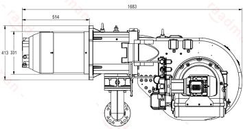
Suggested boiler flange diameter = 343 mm
