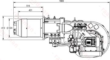
Suggested boiler flange diameter = 343 mm
