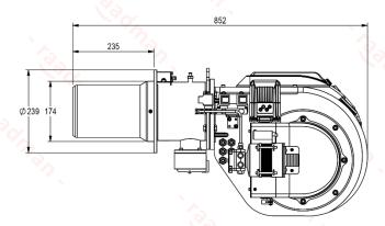
Suggested boiler flange diameter = 186 mm
