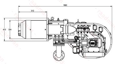
Suggested boiler flange diameter = 346 mm
