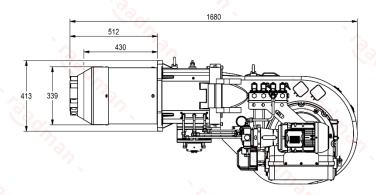
Suggested boiler flange diameter = 346 mm
