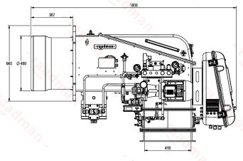
Suggested boiler flange diameter = 492 mm
