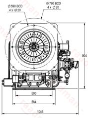
Suggested boiler flange diameter = 492 mm
