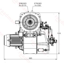
Suggested boiler flange diameter = 492 mm
