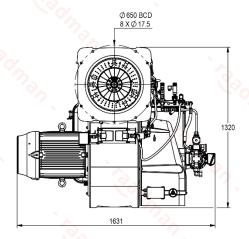
Suggested boiler flange diameter = 492 mm
