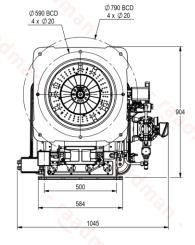
• Suggested boiler flange diameter = 495 mm
