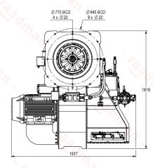
Suggested boiler flange diameter = 620 mm
