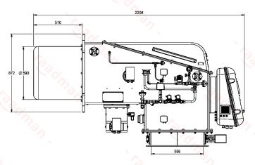
Suggested boiler flange diameter = 602 mm
