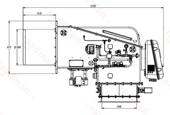
• Suggested boiler flange diameter = 605 mm
