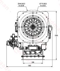
Suggested boiler flange diameter = 620 mm
