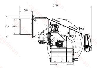
Suggested boiler flange diameter = 620 mm
