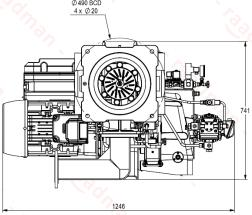
Suggested boiler flange diameter = 348 mm
