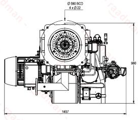
• Suggested boiler flange diameter = 415 mm
