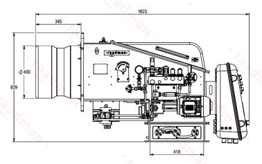
Suggested boiler flange diameter = 415 mm
