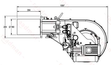
Suggested boiler flange diameter = 192 mm
