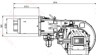
Suggested boiler flange diameter = 235 mm
