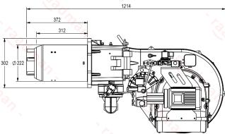
Suggested boiler flange diameter = 235 mm
