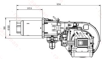
Suggested boiler flange diameter = 235 mm
