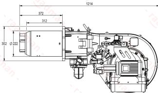
Suggested boiler flange diameter = 235 mm
