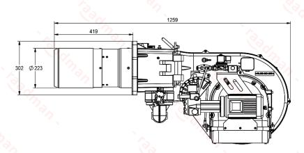
• Suggested boiler flange diameter = 235 mm
