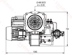
• Suggested boiler flange diameter = 341 mm
