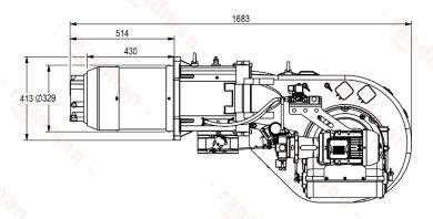
Suggested boiler flange diameter = 341 mm
