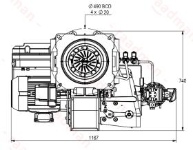
• Suggested boiler flange diameter = 352 mm
