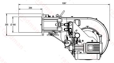
Suggested boiler flange diameter = 202 mm
