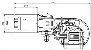
Suggested boiler flange diameter = 235 mm
